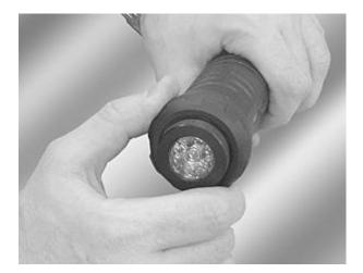
3 Take the LED flashlight out;4 Take the battery out from the handle;5 Connect the ACD to the battery socket;6 Place the ACD in the socket;
