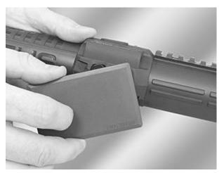
After that the system switches to the Identifiers Programming mode: all identifiers are erased from the system's memory, indicator starts blinking orange. STEP 6. Take the Master-card away from the device. The indicator will keep blinking orange for 10 seconds.
