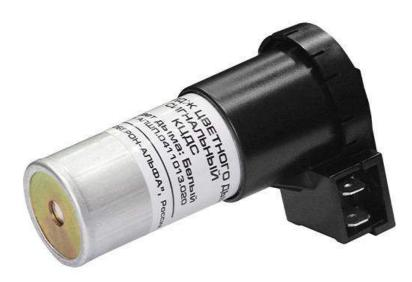
Signal color smoke cartridge (SCSC) is activated with an accumulator battery or any other current source Imin=0.5A; U=6...27V.
